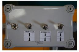
ELECTRO-HYDRAULIC CONTROL UNIT FOR ROTATING THE BAIL, LIFTING SHOE AND DEFLECTOR FLAP
