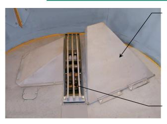
LIFTING SHOE ACTUATED BY HYDRAULIC CYLINDER PREVENTS JAMMING AND FACILITATES STARTING
